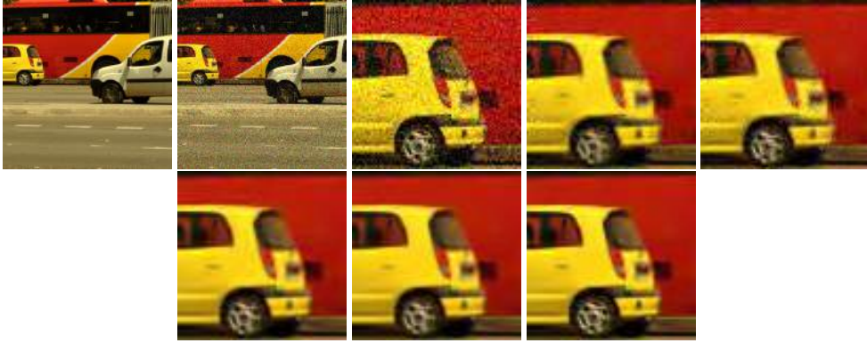
Figure 2.1. Original and noisy images with additive Gaussian white noise; crops of denoised images by Algorithm 1 when incrementally adding the use of a Y_oU_oV_o colour system, uniform aggregation of the 64 estimated values at each pixel, statistically optimal aggregation of the same estimates, and iteration of the Wiener filter with the “oracle” given by the first step. Image quality and SNR increase significantly at each step.
